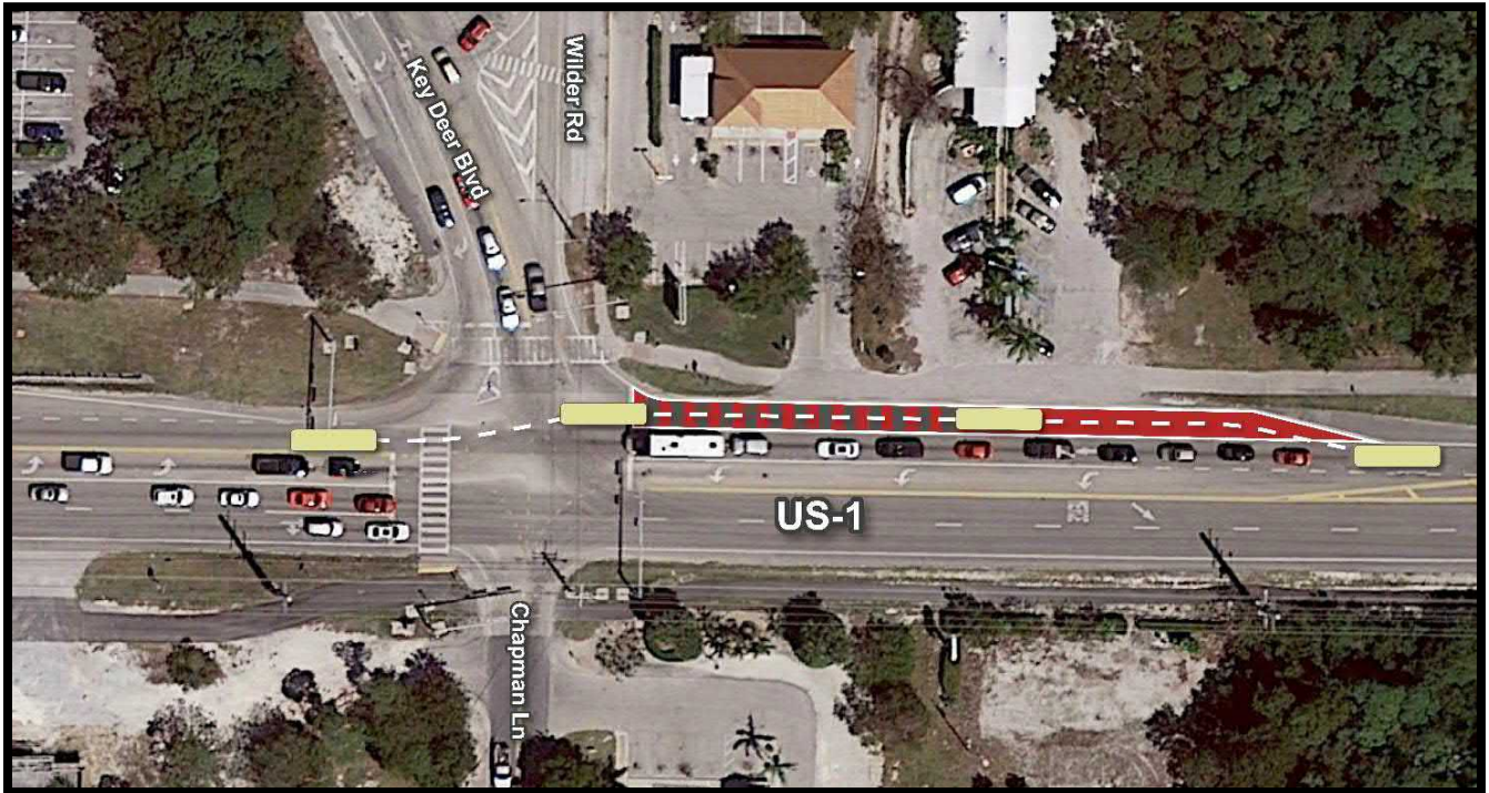
Figure 6-13: Example of potential Queue Jump with Right Turn Lane, Intersection of US 1 and Key Deer Boulevard, Big Pine Key
